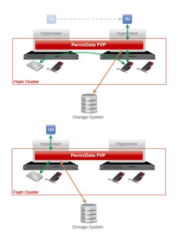
Figure 4 shows how when a VM migrates from one host to another it does not drop its server-side flash footprint for its read and write operations. Instead it simply goes over the backplane to access data on the remote flash (green arrow). This is usually much faster than accessing SAN for the data.
