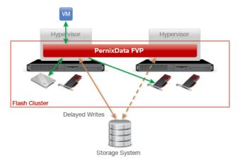
Figure 3 illustrates how data is replicated across the cluster when a VM is configured in Write Back mode. The green arrows indicate how when the VM issues a write operation data it is both written to the local server-side flash and replicated to remote hosts.
