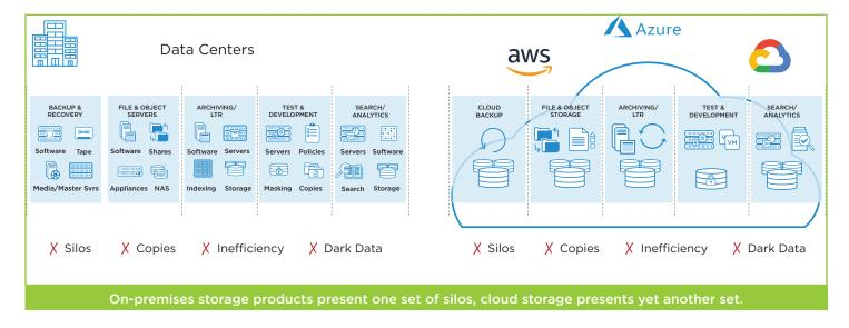
Legacy storage products were not designed to manage data in hybrid cloud environments. On-premises data center storage consists of point solutions such as NAS appliances, deduplication appliances, archive storage and analytics clusters. Cloud storage presents another, different set of silos including object, file and cold archive storage.
